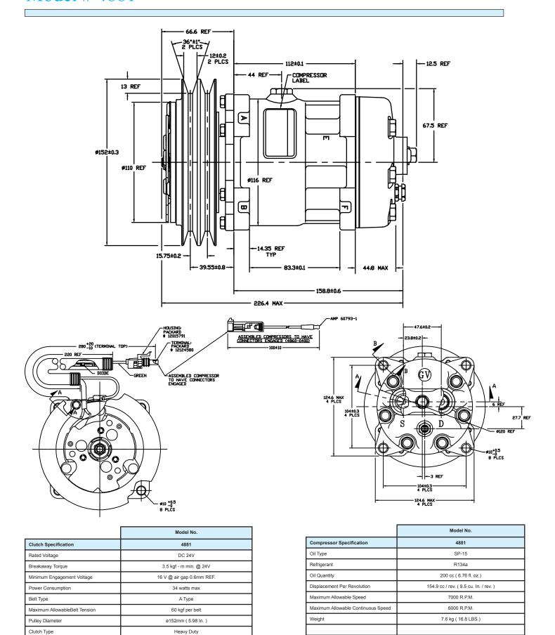
Note: Models with 24 volt clutch have 280mm, green lead wire.
