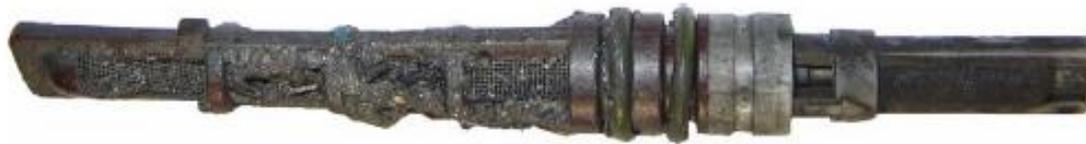
Example of contamination collected on inlet side of orifice tube requiring system flushing
