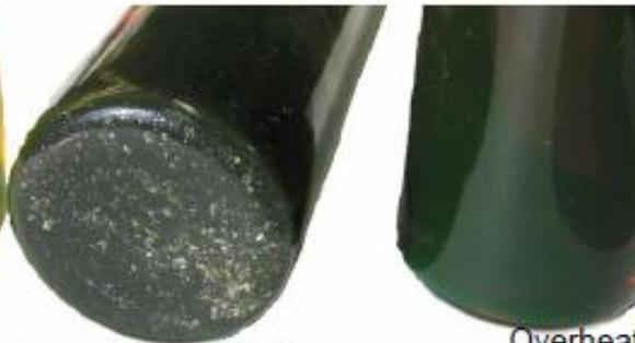
Contaminated oil with metal particles will require system flushing
