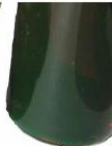
Overheated oil is dark and will require flushing
