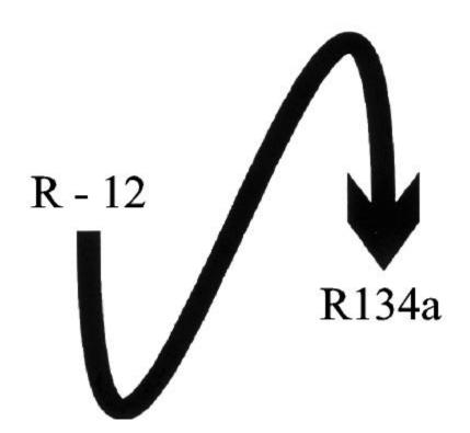
The use of R134a in mobile A/C systems designed for R-1 2 refrigerant causes higher discharge pressures (as much as 10-15%) and necessitates changing the compressor lubricant from mineral oil (5GS) to PAG oil (Sanden's SP-10 or SP-20) to ensure compatibility.
